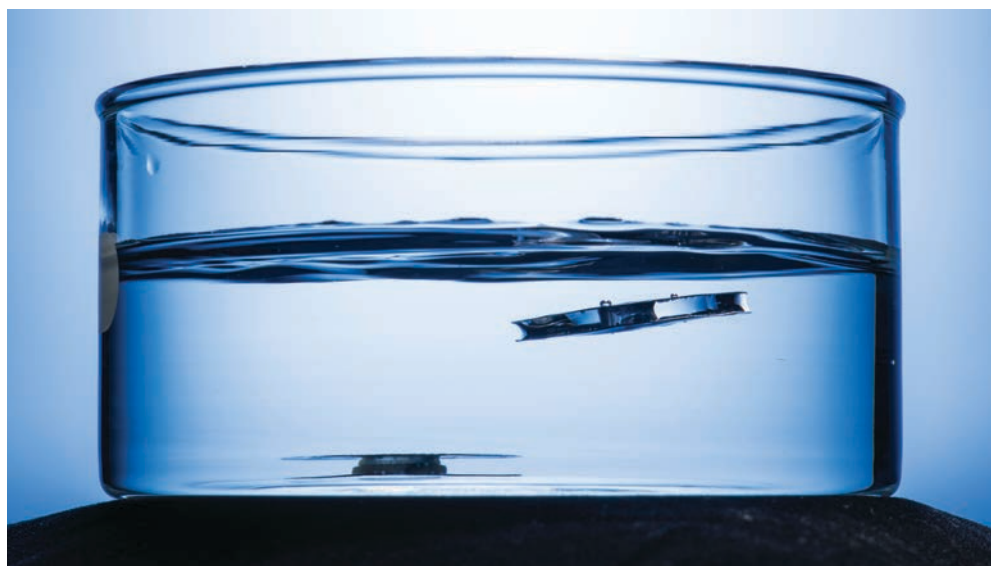
FLOAT YOUR BOAT? A metal structure treated with extremely brief, high-powered laser bursts rises to the surface compared to an untreated disc, part of Rochester research to explore how lasers interact with metal.
