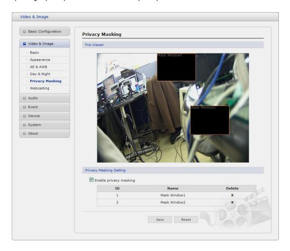
The privacy masks are configured by Mask windows. Each window can be selected by clicking with the mouse. It is also possible to **resize or delete, or move** the window, by selecting the appropriate window at the mouse menu on the video screen.
