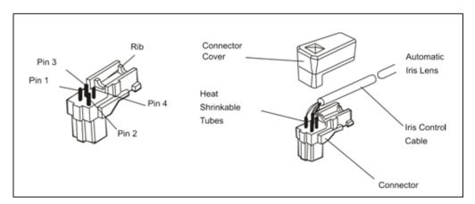
1. Solder the lens control wires to the connector supplied with the camera.
