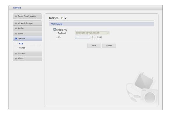
The Network Camera supports several PTZ devices. Using an appropriate cable, connect the device to your RS-485 port. These ports are available via the I/O terminal connector.
