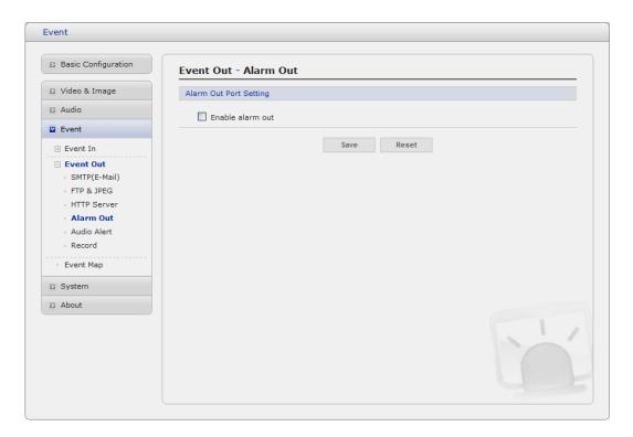
When the network camera detects an event, it can control external equipment connected to its alarm output port. Check the box to enable and then select either:
