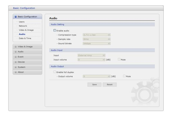
The Network Camera can transmit audio to other clients using an external microphone and can play audio received from other clients by attaching a speaker. The Setup page has an additional menu item called **Audio**, which allows different audio configurations, such as, full duplex, and simplex.
