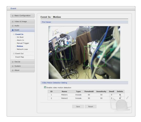
Motion detection is used to generate an alarm whenever movement occurs (or stops) in the video image. A total of 8 Motion and/or Mask windows can be created and configured.
