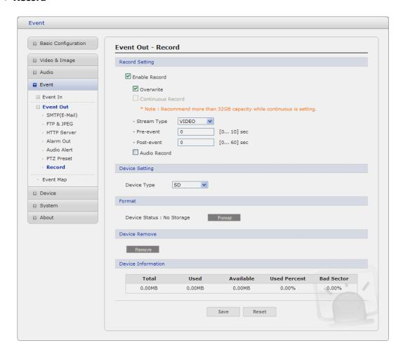
When the network camera detects an event, it can record video stream in the Micro SD Memory (not supplied) or NAS (Network Attached Device) as a storage device. Check the Enable record checkbox to enable the service.
